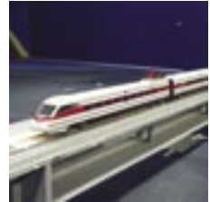
Wind tunnel tests on a model of a High Speed train, to define the effect of crosswinds on ride safety
