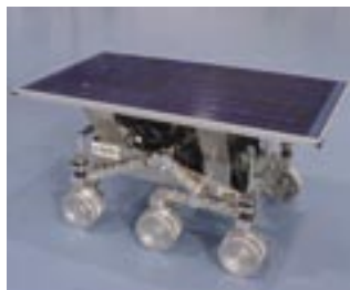
CASIMIRO (Cheap Automated Stereo Images Environment Identification Rover), a six wheels rover for space exploration developed at the Dept. of Aerospace Engineering of the Politecnico di Milano
