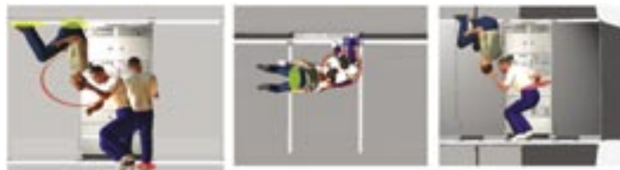
Study of a restraint to be used during experiments' performance in microgravity inside the Columbus Laboratory, International Space Station (research "MEEMM Operational study" for ESA - European Space Agency). From the doctoral thesis in Industrial design and Visual Communication: "Habitability in space: Design for microgravity"
